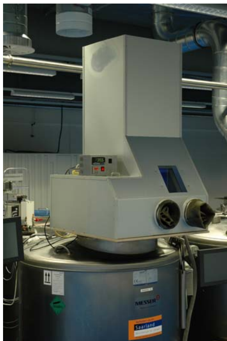
Fig. 1: Access tower on Cryotank.
