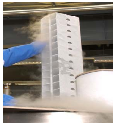
Fig. 2: »Classic« sample extraction with months of ice formation on the surfaces (substrate, container, tank interior) and interruption of the cooling chain.
