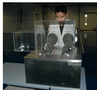
Fig. 4: Cover technology for contamination-free handling. The cover-cooler systems can be cooled either manually or automatically by liquid nitrogen in an absorbent matrix for hours. From bottom to cover a stable temperature gradient develops from -196\text{ °C} below to +20\text{ °C} at the top. Cell samples can such be handled and stored on shelves in different heights at any given temperature. The system is inexpensive and can be extended to a parallel freeze/thaw automat. It is a basic device for future cryolaboratories.
